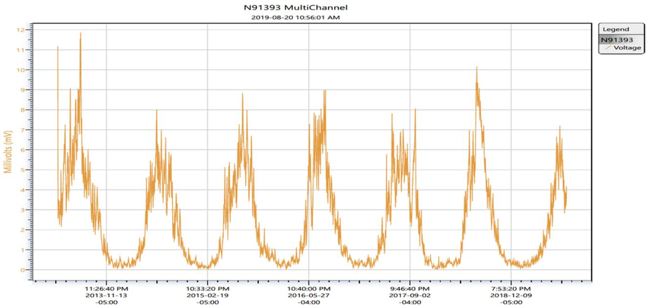
Figure 8 Monitoring galvanic current
